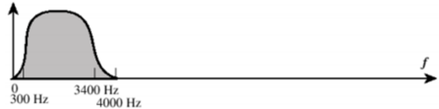
(a) Each voice channel is bandlimited between 0.3 – 3.4 KHz
